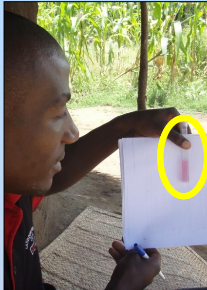
Positive test for chlorine in stored water
